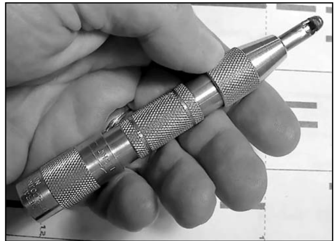
Figure 12. A hand-made, hollowed-out center punch.
