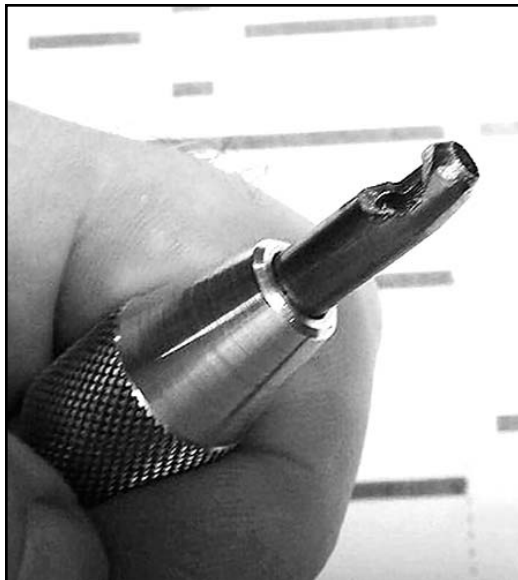
Figure 13 (above). A finished hollowed-out center punch.
